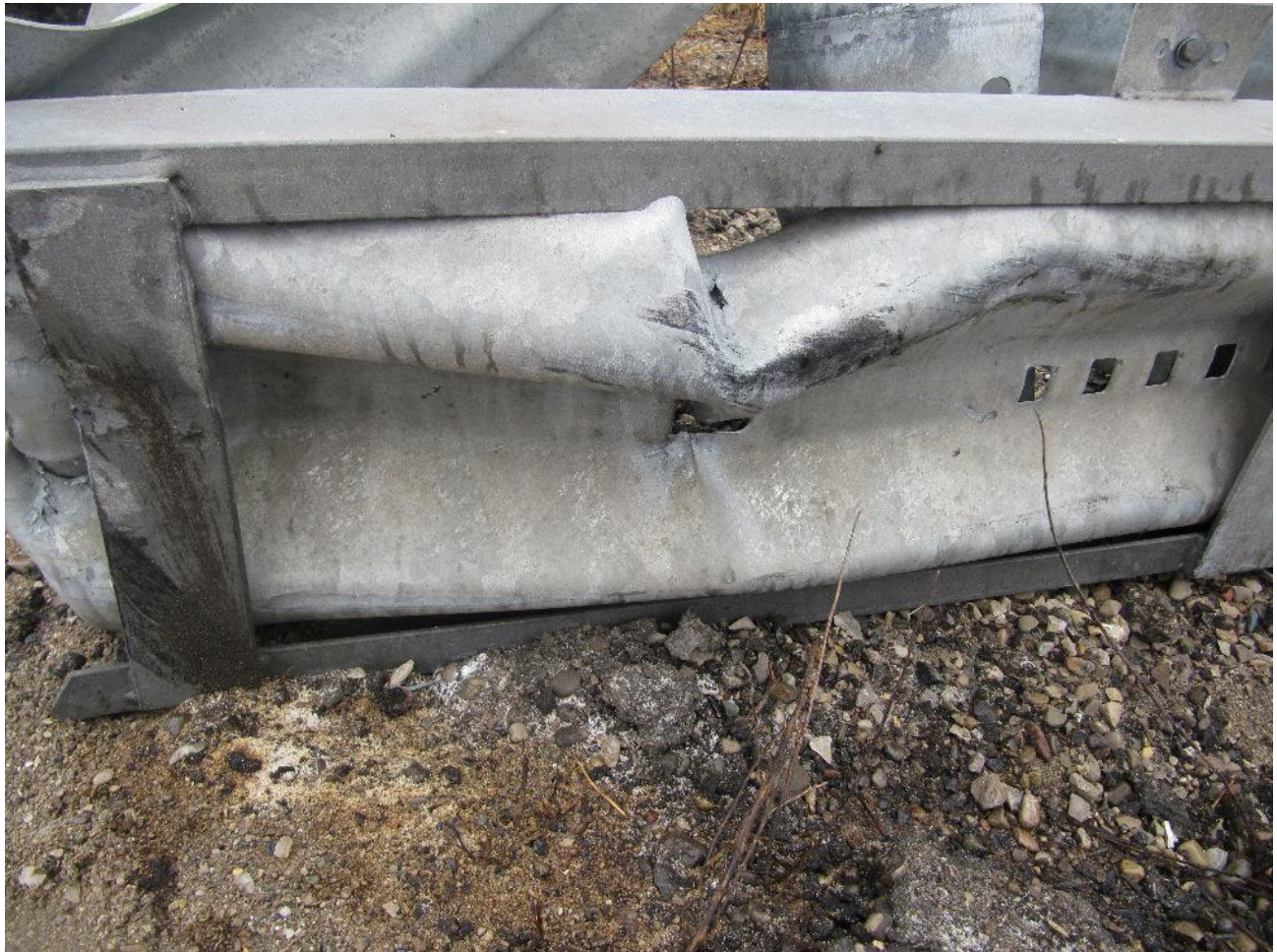
Figure 17: View of buckling of the rail while resting within the channel.
