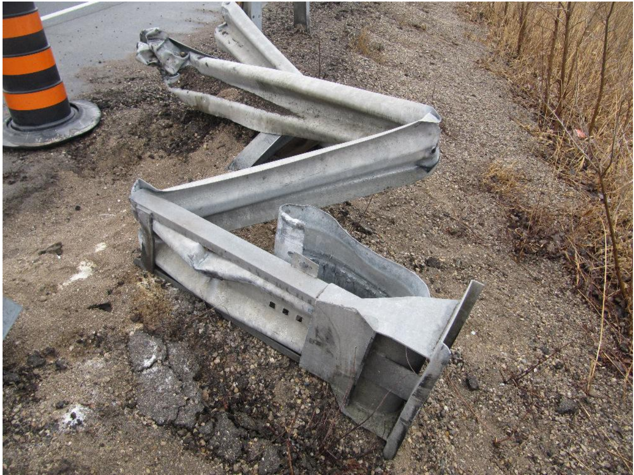
Figure 14: Overall view of buckled guardrail and a short length of rail that has been extruded out the side of the terminal head.
