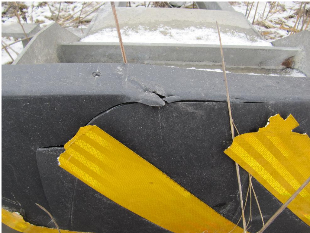
Figure 26: View of the minor tears to the cover of the head (impact plate) confirming that an actual impact occurred to the unit.
