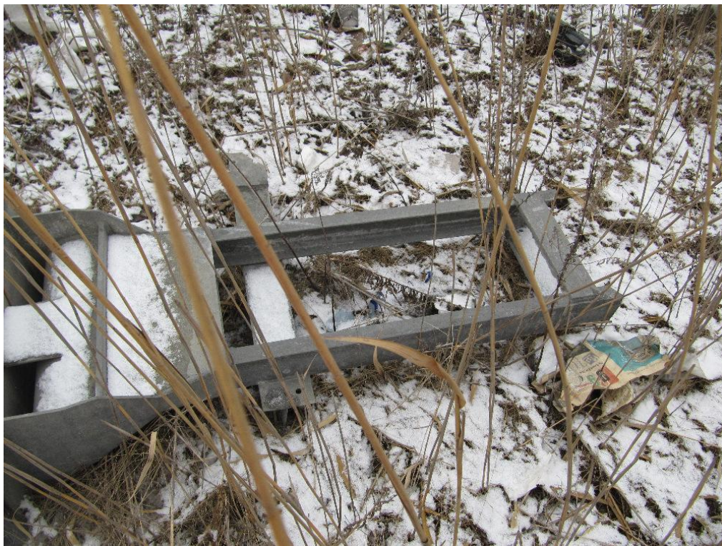
Figure 24: Note the lack of any structural deformation to the terminal.
