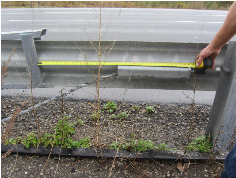
Figure 12: Measurement taken to locate the channel and head with respect to the guardrail.
