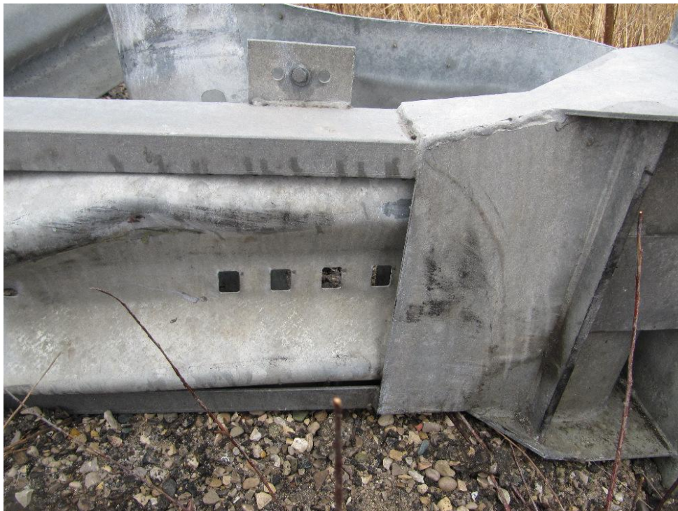
Figure 16: View of anchorage holes in the rail where the teeth of the anchorage bracket would have fit. This indicates the extent of travel of the rail through the head as a result of the impact.
