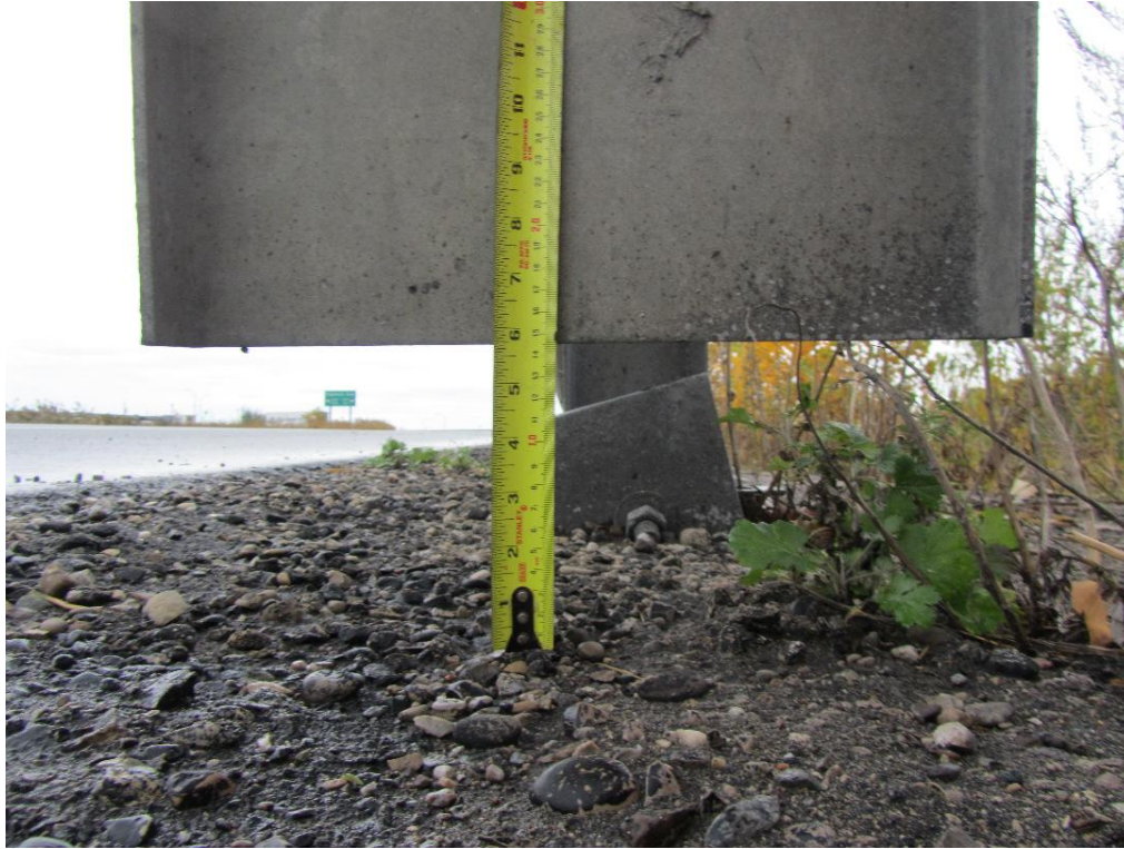
Figure 9: Measurement of the installation height of the terminal head during an inspection on October 14, 2014.
