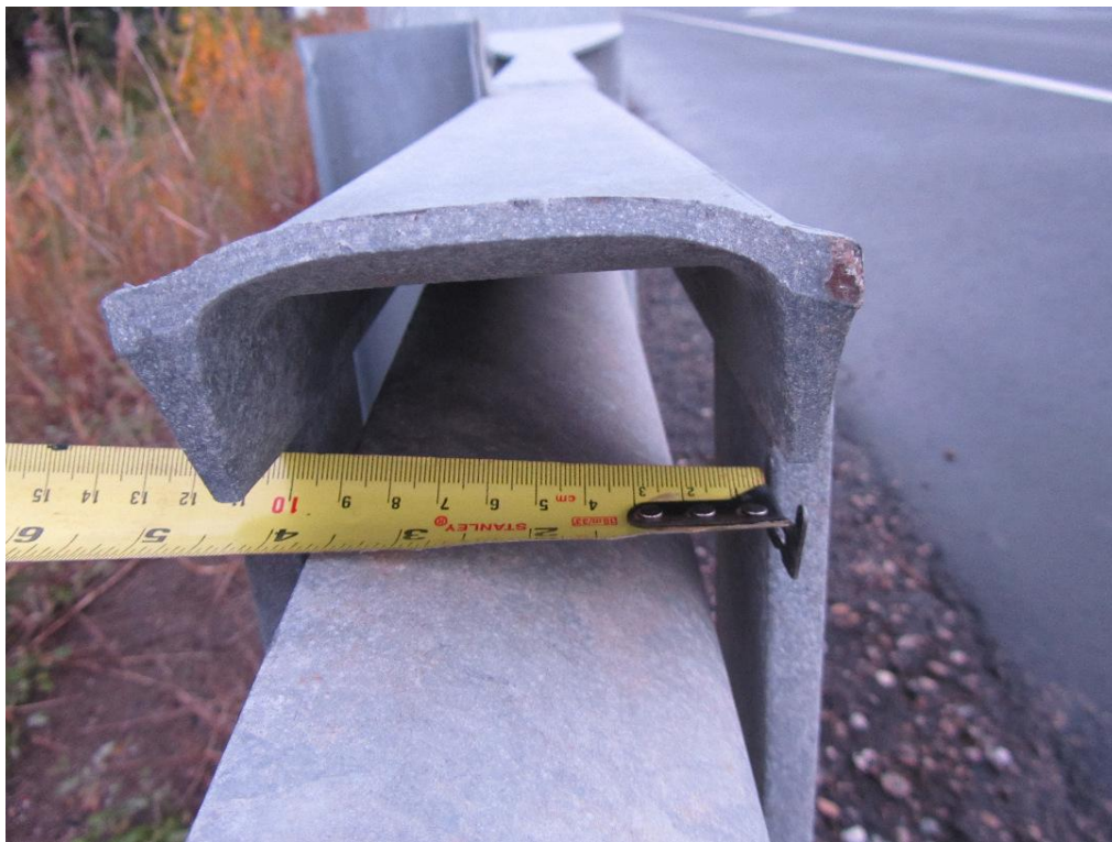
Figure 10: Measurement confirming the 4-inch-wide channel of the ET-PLUS terminal (Photo taken on October 14, 2014).
