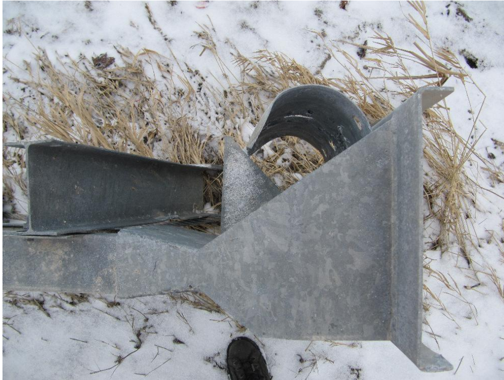
Figure 3: Top view of the ET-PLUS terminal showing how a minor impact has caused the head and channel to be displaced along the guardrail. Consequently the end of the guardrail has been squeezed out the side of the head.
