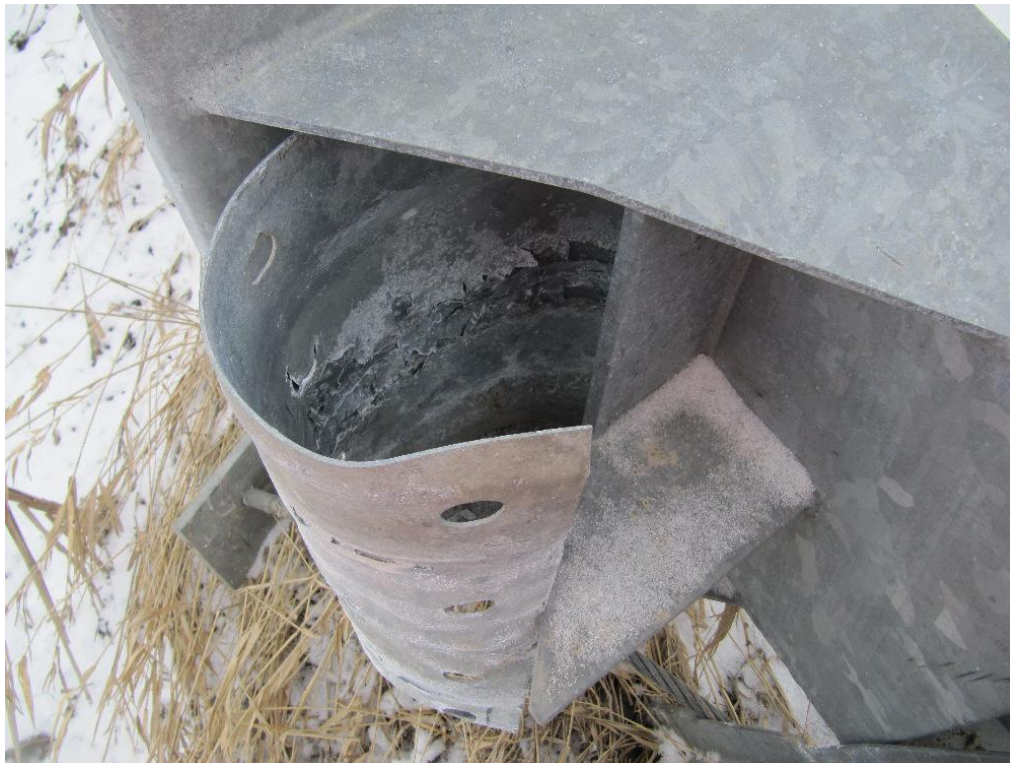
Figure 4: Ditch-side view of the end of the guardrail as it has been squeezed and deformed from passing through the narrow opening in the head.
